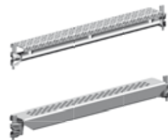
U-gap decks/U-ledgers with gap cover , 0.11 m wide are available in a variety of lengths for gap-free work surfaces between U-main scaffolding decks and U-console bracket decks (see pages 42 / 43).
